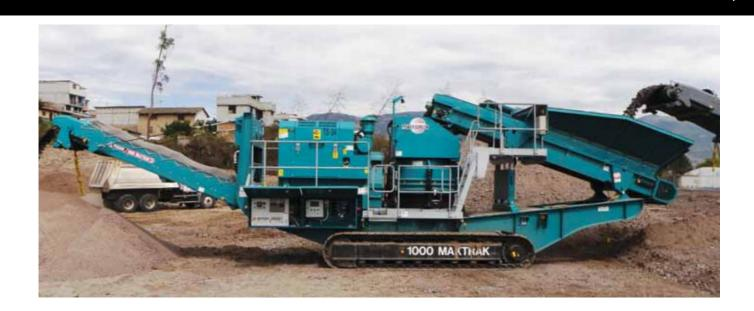
The high performance Powerscreen® 1000 Maxtrak is a small to medium sized cone crusher which has been designed for direct feed applications without pre-screening on clean rock. At its heart is the Automax® cone crusher which provides excellent reduction and product cubicity for the production of high quality aggregate and sub-base material. Hydraulic release capabilities are designed so that any uncrushable material entering the chamber is safely discharged.
